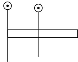
Moment of inertia about an axis passing through one end =  $I_{cm} + md^2$
